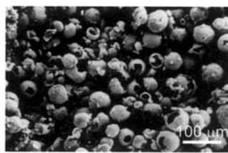
FIGURE 4. SEM photograph of \text{Al}_2\text{O}_3 -5.0 wt% \text{SiO}_2 hollow microspheres.
